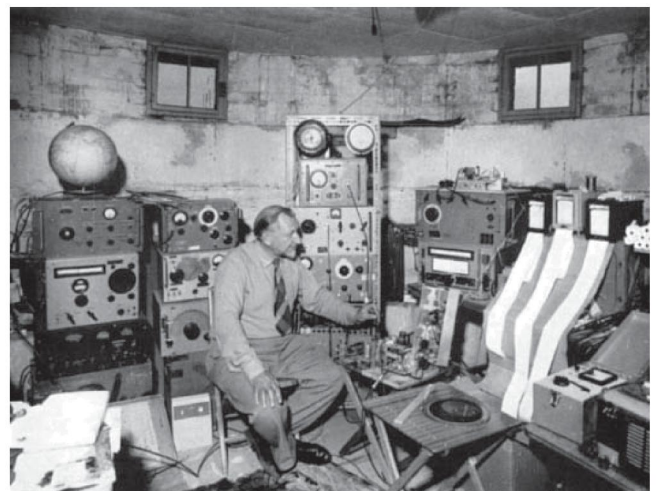
Figure 6. Hyde's Martello Tower radio telescope control room, which he called 'the eyepiece'. Note the pen recorders and charts, funded via Carnegie grants to the BAA. From Radio Astronomy for Amateurs .
