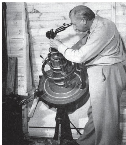
Figure 10b. The eyepiece end of the 9-inch Coudé inside Hyde's wooden building. The spectroscope Hyde is using is BAA Instrument No. 8. From Radio Astronomy for Amateurs .
